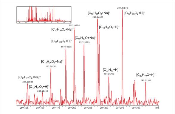
**Figure 2.** EBC positive mode mass spectrum with  $> 10\,000\,m/z$  peaks in top left. Zoom into nominal mass 297 with corresponding ion formula assignments of m/z peaks.
