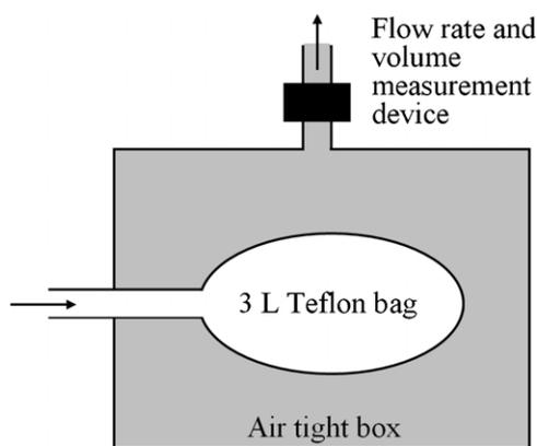
**Figure 1.** Setting for measuring the breath volume and flow rate.
