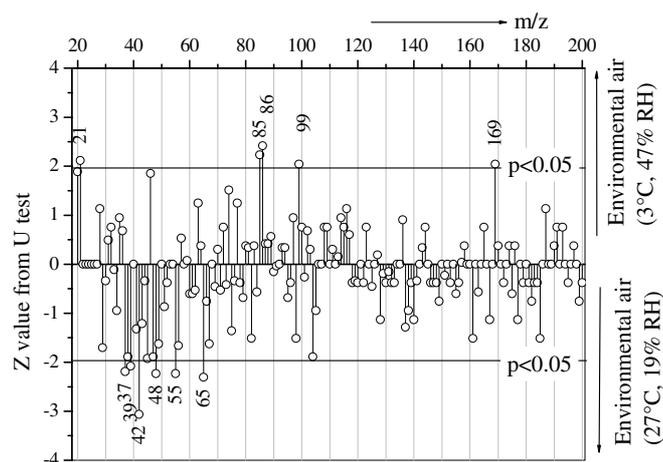
**Figure 2.** *U*-test between the concentrations of exhaled VOCs sampled after a 5 min stay under two different surrounding air conditions ( $n = 10$  volunteers).
