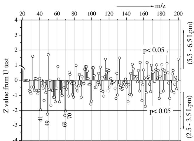
**Figure 4.** U-test between the concentrations of exhaled VOCs sampled with high (5.5–6.5 L min<sup>-1</sup>) and low (2.5–3.5 L min<sup>-1</sup>) breathing flow rates (*n* = 10 volunteers).
