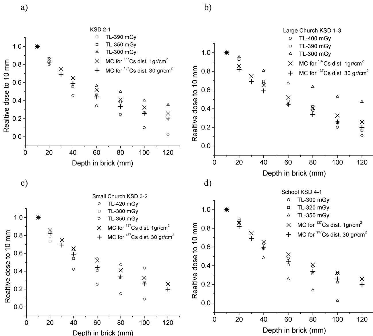
**Fig. 3.** Relative depth-dose distribution obtained using MC simulations and  $D_T$ - $D_{BG}$  curves plotted for incremental variation of  $D_{BG}$  values. The best fits were obtained a) at 350 mGy for sample KSD-2-1, the Large Church, b) at 390 mGy for sample KSD-1-3, the Large Church, c) at 380 mGy sample KSD- 3-2, the Small Church, and d) at 320 mGy for sample KSD-4-1, the School.
