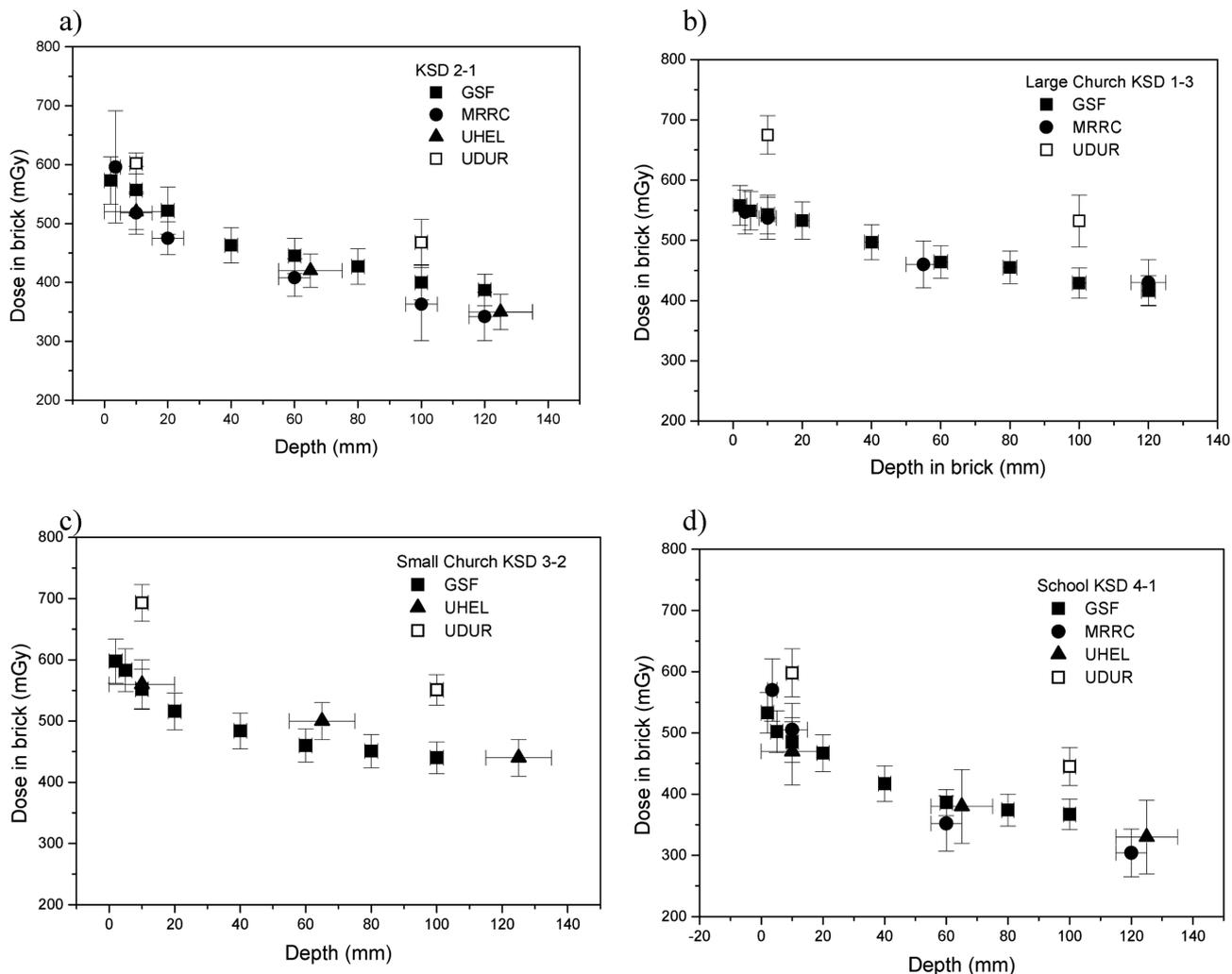
**Fig. 2.** Graphical representation of the depth-dose distribution measured using TL and OSL for various sections of a brick from a) the Large Church, sample KSD-2-1; b) the Large Church, sample KSD-1-3; c) the Small Church, sample KSD-3-2 and d) the School, sample KSD-4-1.
