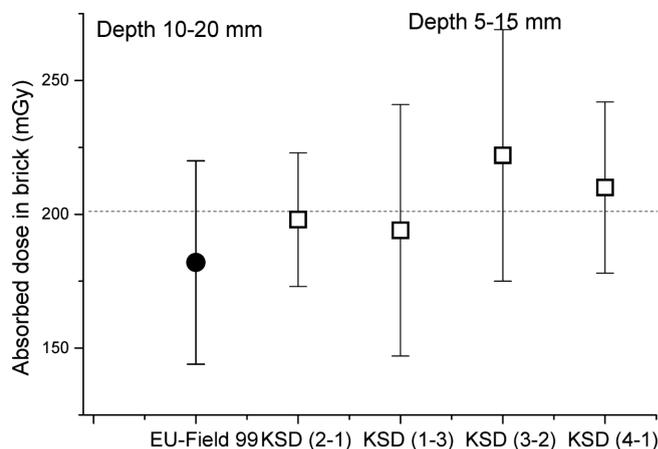
**Fig. 4.** Comparison of fallout dose in brick collected at a height of 1 m above ground at Dolon’ in 1999 by the EU supported Measurements Group to those obtained from bricks at unknown height distributed for the intercomparison measurements.
