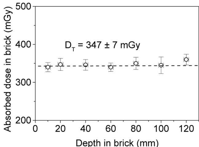
**Fig. 1.** Depth-dose profile in a brick collected from an inner wall of the former Large Church.
