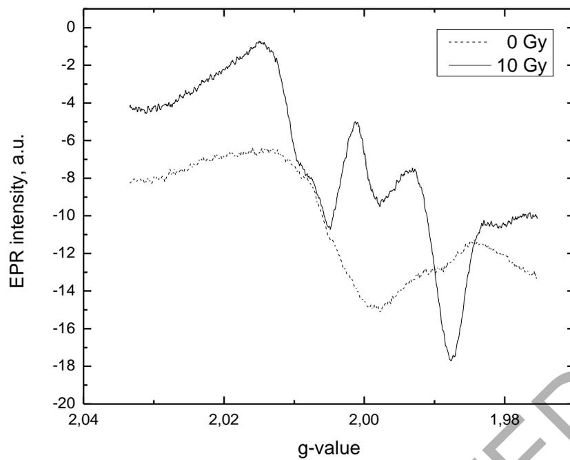
Figure 2: EPR spectra of unexposed and 10 Gy exposed Gorilla glass samples.
