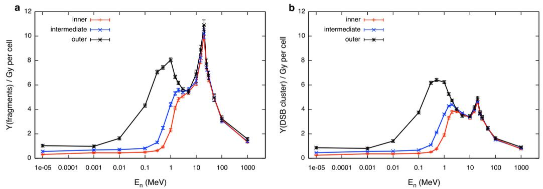
**Figure 7. Variation with neutron energy and location in the phantom of neutron induced DNA damage.** Neutron induced DNA damage: (a) DNA fragments shorter than 30 bp; (b) DSB clusters; damage per Gy per cell as a function of neutron initial energy in the three scoring regions in the phantom. Lines are drawn to guide the eye. Error bars come from standard deviations among results on doses of secondary species for batches in a single run as given by PHITS.
