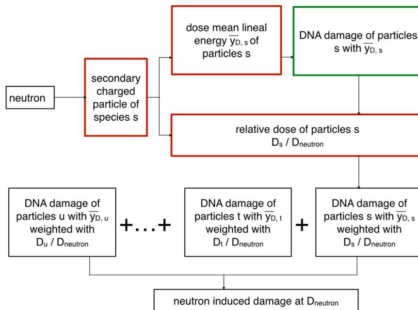
**Figure 6. Proposed coupling scheme for transport and track structure results.** Calculation scheme followed for the coupling of transport (PHITS) and track structure calculations (PARTRAC) to obtain neutron induced DNA damage. Red boxes identify information from PHITS, green boxes information from PARTRAC. Details are given in the text.
