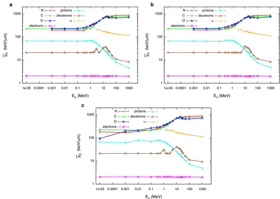
**Figure 3. Variation with neutron energy and location in the phantom of the dose mean lineal energy of secondary charged species.** Dose-mean lineal energy values for secondary charged species accelerated by neutrons as a function of neutron initial energy: (a) inner; (b) intermediate; (c) outer scoring region. Error bars are standard deviations among different PHITS runs and are in most cases within the symbols. Lines are drawn to guide the eye.
