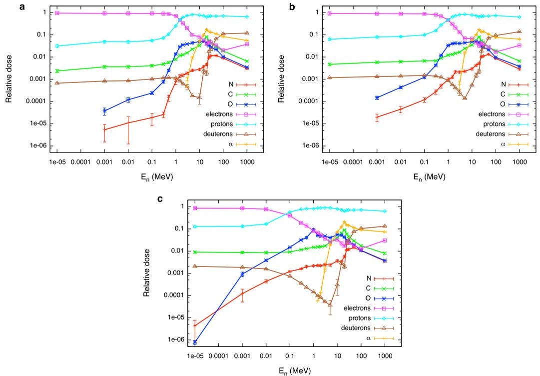
**Figure 2. Variation with neutron energy and location in the phantom of the relative contribution of secondary charged species to the total neutron dose.** Relative contributions of secondary charged species to the total neutron dose as a function of neutron initial energy: (a) inner; (b) intermediate; (c) outer scoring region. Error bars are standard deviations among results for batches in a single run as given by PHITS. Lines are drawn to guide the eye.
