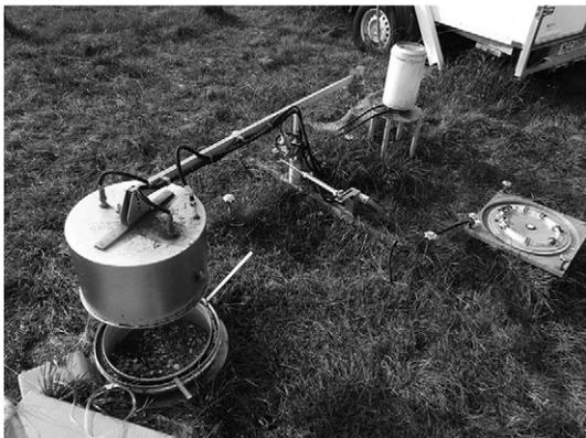
Figure 1. Exhalometer set-up in operation.
