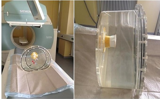
**Fig. 1** Siemens Symbia T6 SPECT-CT with NEMA IEC body phantom filled with water including a vial with 25 ml volume (calibrated activity of 651 MBq).
