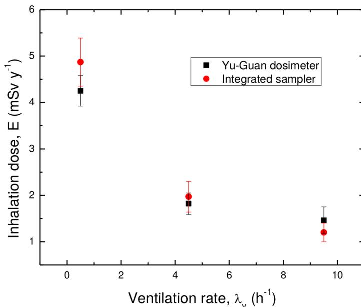
**Figure 5.** Variation of inhalation dose,  $E$  ( $\text{mSv y}^{-1}$ ) with increase in ventilation rate measured with Yu-Guan dosimeter and Integrated sampler.
