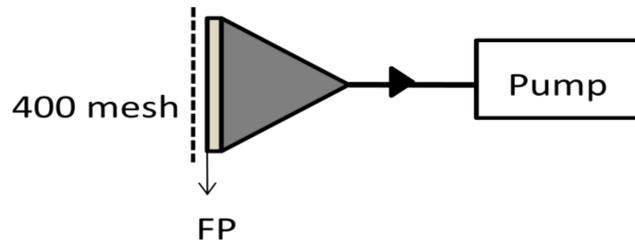
**Figure 1.** Schematic diagram of the Yu-Guan dosimeter (YG).
