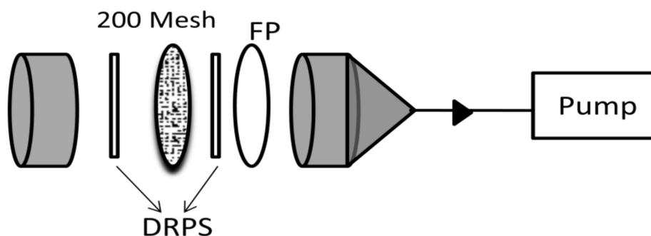
**Figure 2.** Schematic diagram of integrated sampler (IS) using wire mesh and filter paper which face the direct radon progeny detectors (DRPS).
