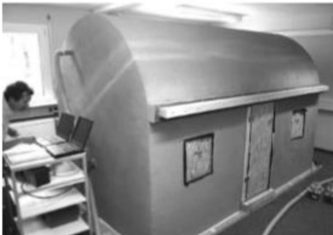
**Figure 3.** Thoron experimental test house, HMGU, Germany.
