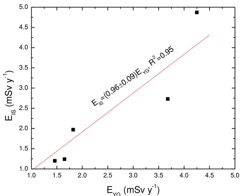
**Figure 4.** Correlation between inhalation dose,  $E$  ( $mSv\ y^{-1}$ ) measured with Yu-Guan dosimeter and Integrated sampler.
