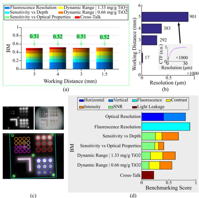
**Fig. 5. Validation of phantom-based benchmarking of surgical microscopy and raster scan systems.** (a) Individual BMs for raster-scan System 3. (b) Fluorescence resolution as a function of working distance for System 3. The inset shows the contrast transfer function vs resolution at a working distance of 5 mm. (c) Fluorescence (top left) and color (top right) images acquired from System 5. Phantom elements are segmented (bottom) for further analysis. (d) Individual BMs for System 5.
