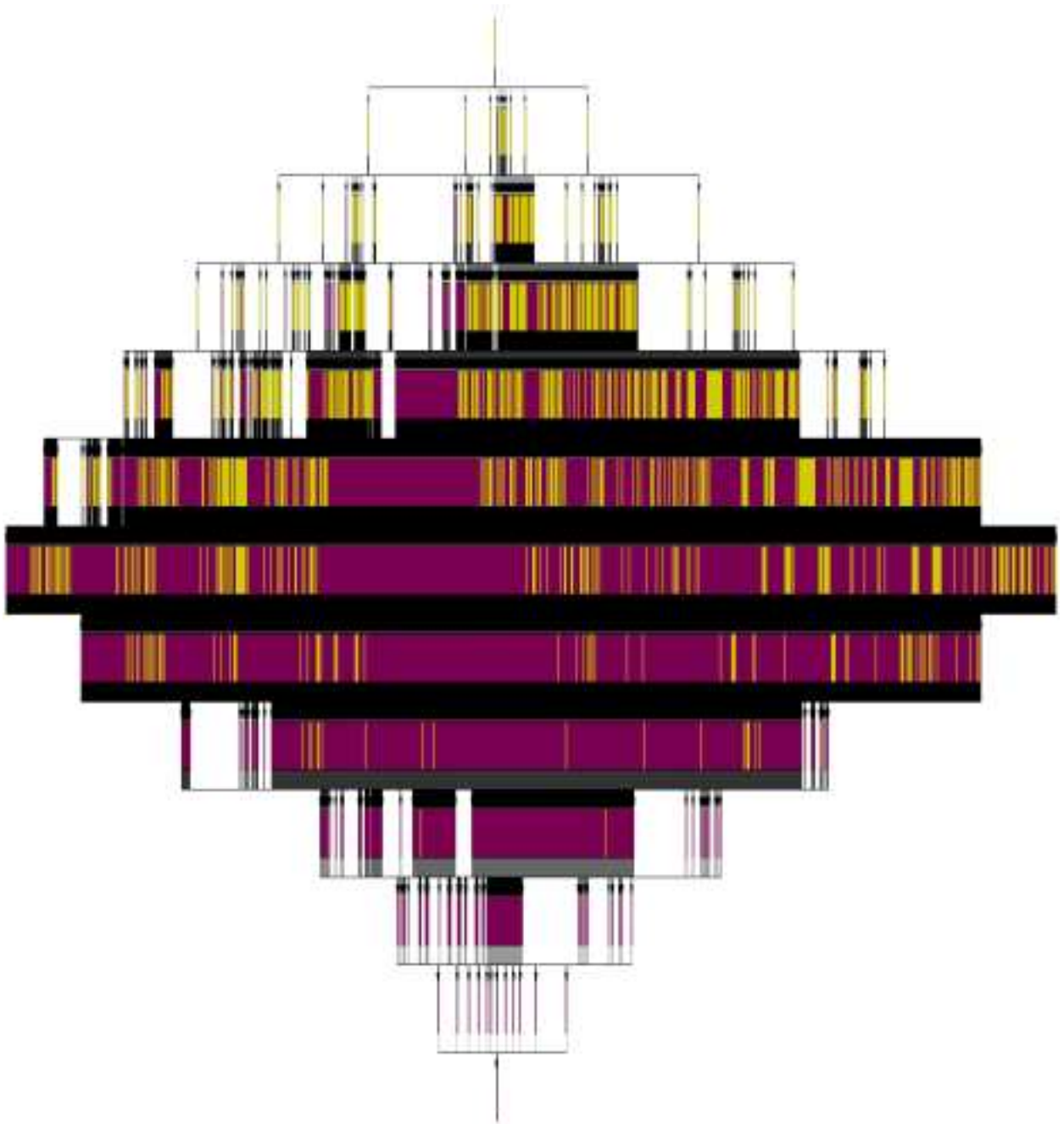
Figure 7.2.: Complete reduction graph of the artificial model employed; yellow states are valid, violet states are invalid.
