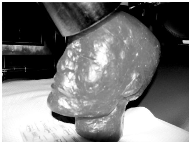
**Fig. 2.** Counting the BfS phantom at the forehead contact position ("Position 1") using the HML lung counter.
